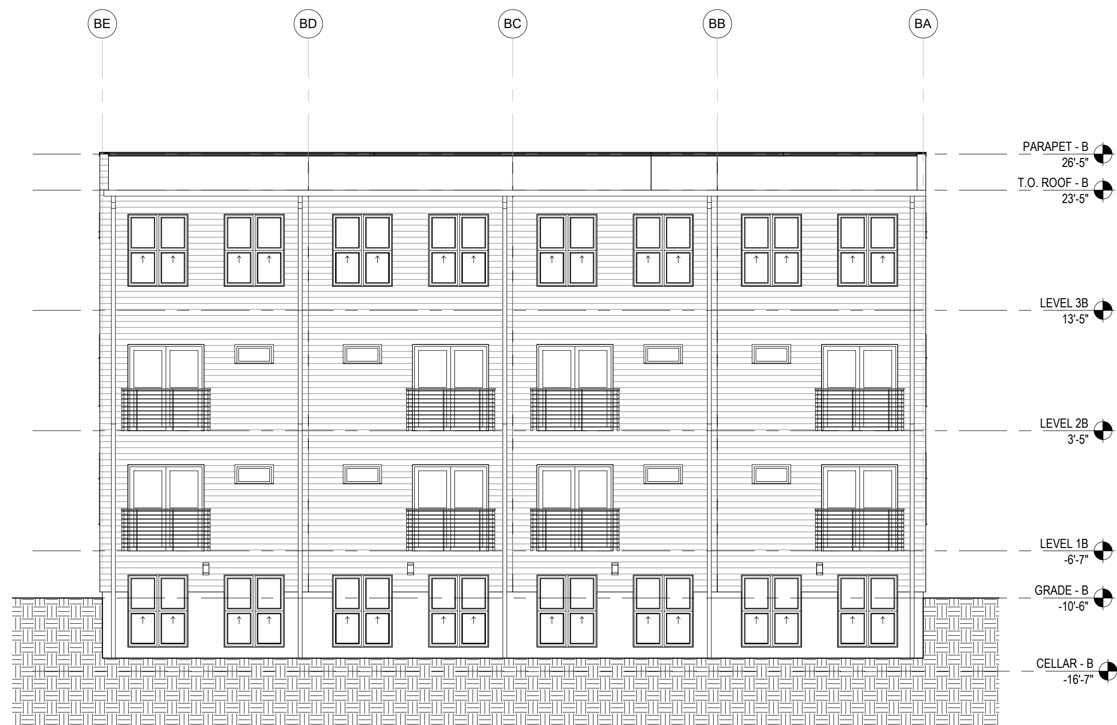
BUILDING B - NORTH ELEVATION 2 1/8" = 1'-0" A401
